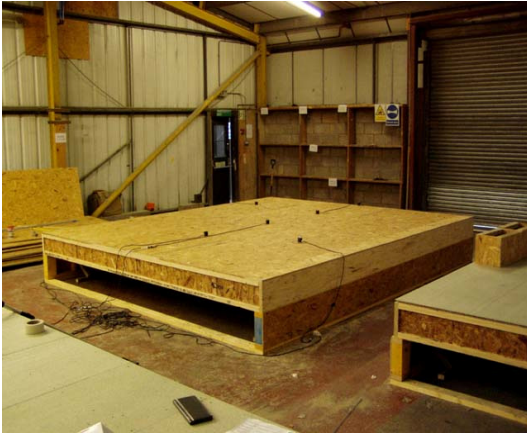
Fig. 1 - Two side supported timber floor prepared for dynamic tests
