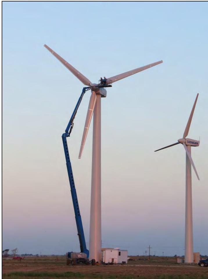
Figure 3. Impact modal testing performed on SNL1.
