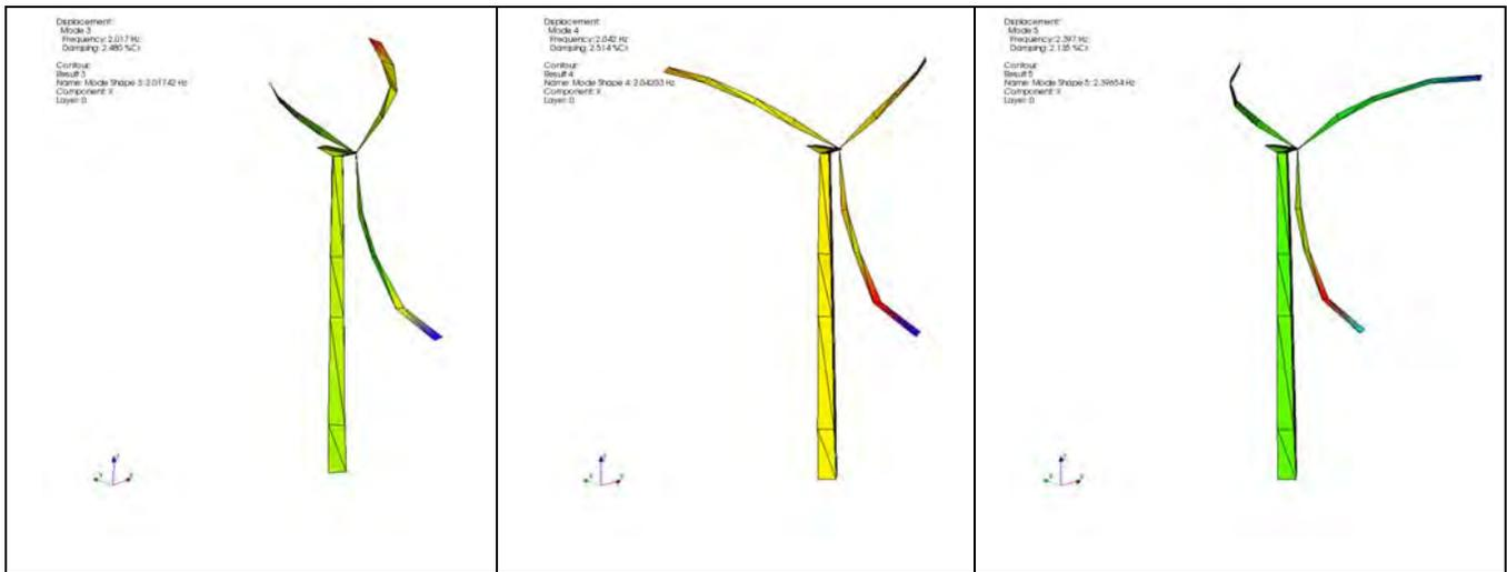
Figure 6. First three flapwise bending modes.
