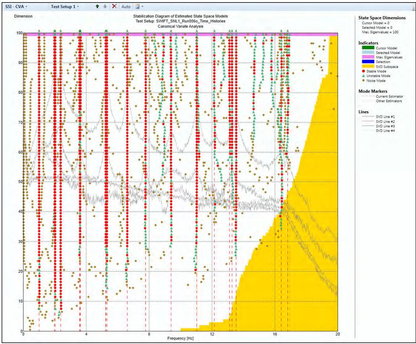
Figure 8. Stability diagram in ARTeMIS for the SSI-CVA algorithm.
