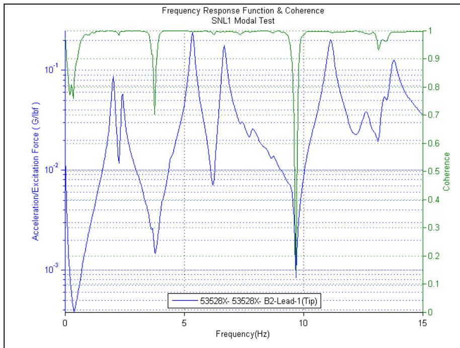
Figure 4. Drive point FRF and coherence from impact on SNL1 blade tip.
