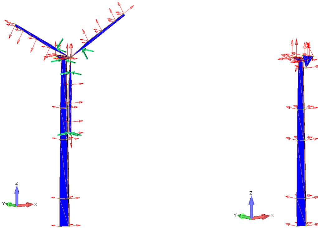
Figure 2. Test display models for SNL1 (left) and SNL2 (right). Green arrows represent excitation locations.
