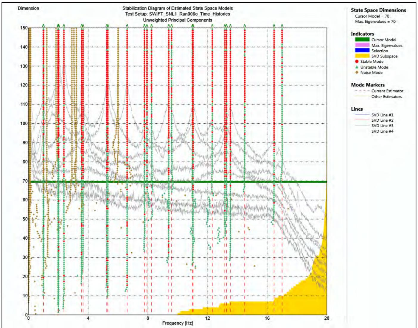
Figure 9. Stability diagram in ARTeMIS for the SSI-UPC algorithm.
