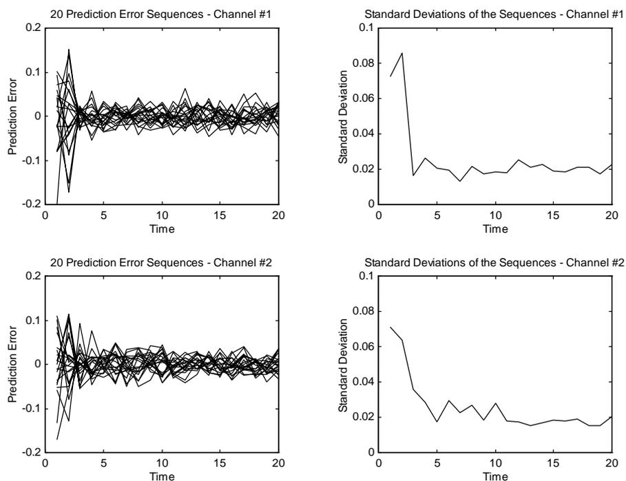
Figure 7.1: Transient behaviour of the prediction errors of an ARMAV(2,2). The left-hand side plots show 20 different prediction error sequences, and the right-hand side plots the variation of the standard deviation of these.
