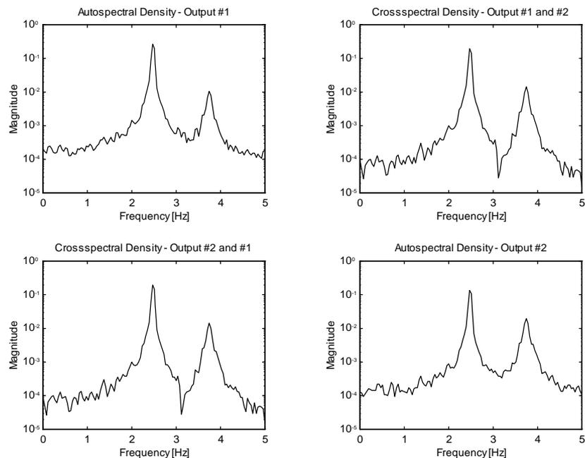
Figure 7.2: Spectral densities of noise-contaminated simulated response.
