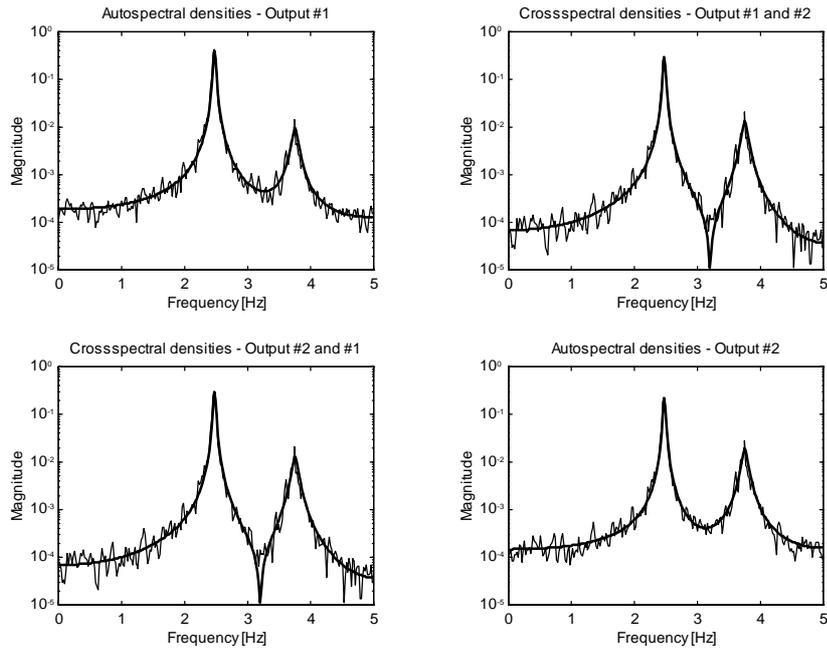
Figure 7.4: Comparison of spectral densities obtained directly from the measured response using FFT and obtained from the estimated model. The smooth lines are the spectral densities of the model.
