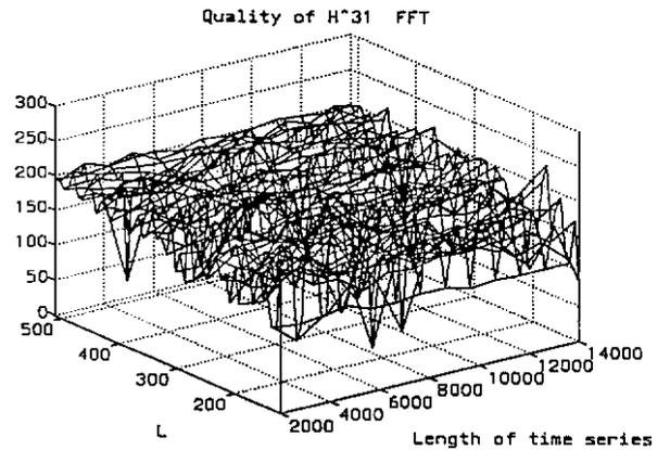
Figure 12: Quality of FRF  $H_{31}$  estimated by FFT.
