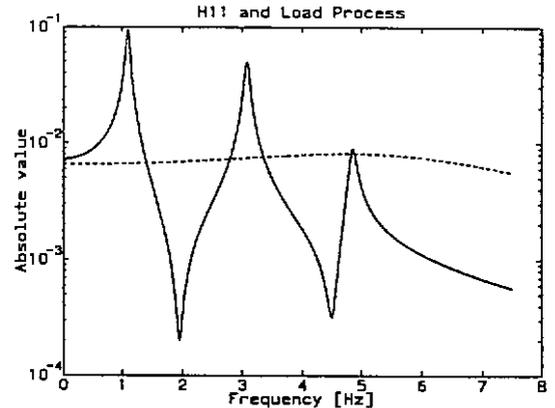
Figure 2: Theoretical absolute value of FRF,  $H_{11}$ , and theoretical absolute value of load applied to mass 1.
