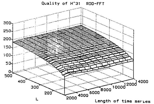
Figure 11: Quality of FRF  $H_{31}$  estimated by RDD-FFT.
