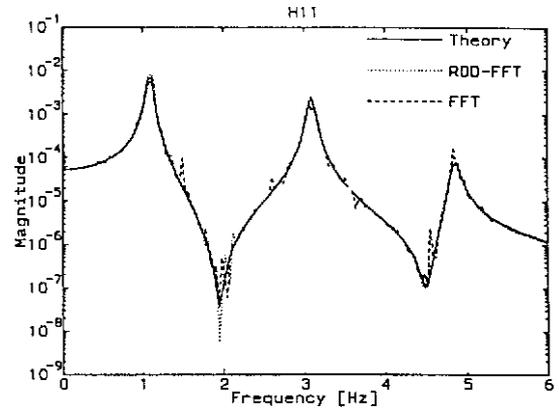
Figure 5: Magnitude of frequency response function,  $H_{11}$ .
