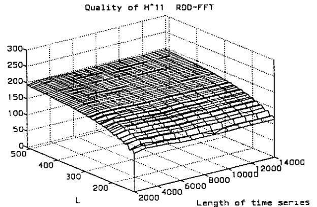
Figure 7: Quality of FRF  $H_{11}$  estimated by RDD-FFT.
