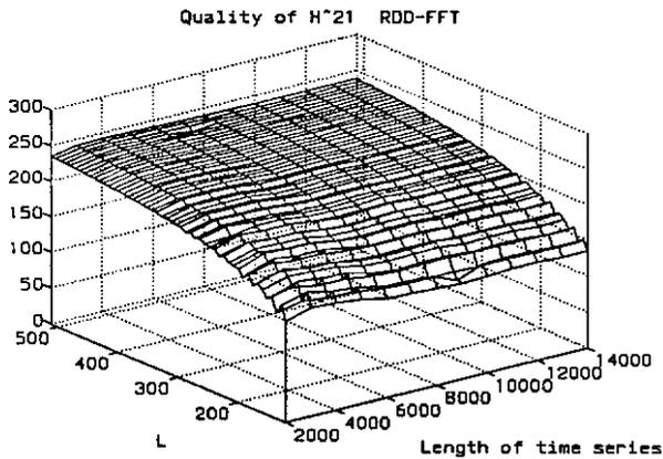
Figure 9: Quality of FRF  $H_{21}$  estimated by RDD-FFT.
