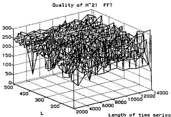
Figure 10: Quality of FRF  $H_{21}$  estimated by FFT.
