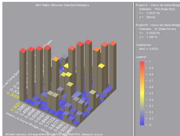
Fig. 7 – MAC matrix plot for mode shapes estimated by FDD and SSI methods
