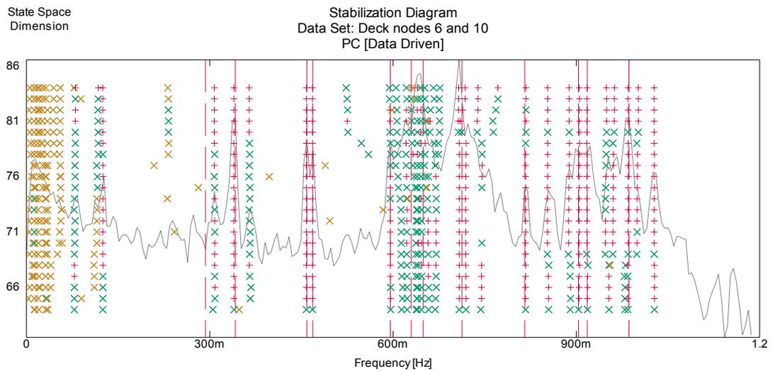
Fig. 6 – Stabilization diagram for data set 6 (measurement sections 6 and 10)
