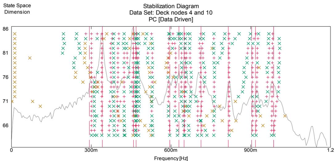
Fig. 5 – Stabilization diagram for data set 4 (measurement sections 4 and 10)
