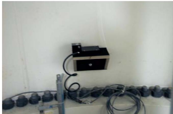
**Figure 10. Accelerometer mount at the connection between the tower and the foundation.**
