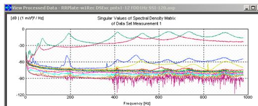
**Figs.4c** SVD with two fixed broadband excitation sources (different points than in 4b)
