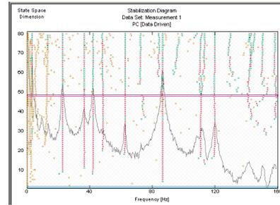
**Fig.9b** Stabilization diagrams with five projection channels
