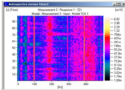
**Fig.2** Example of a contour plot of a STFT of a response signal revealing random as well as sinusoidal content
