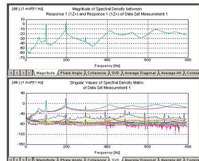
**Fig.6** Autospectrum and SVD plot from a test similar to the one shown in Fig.2
