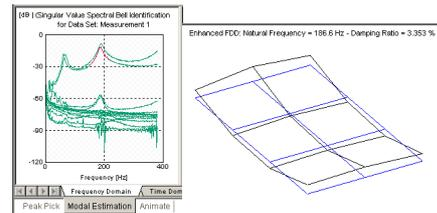
**Figs.5a** Bending mode estimated from the FDD (SVD) shown in Fig 4b
