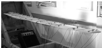
**Fig.1a** Model of wind turbine wing analyzed using acoustical excitation
