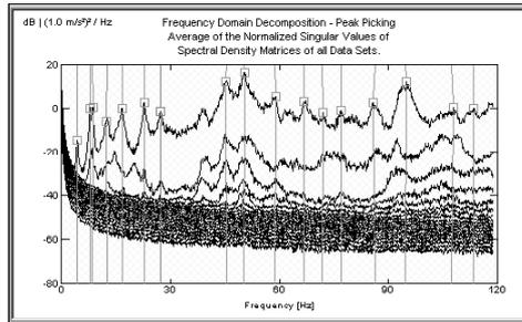
**Fig.3a** SVD plot from the test of the wind turbine wing model
