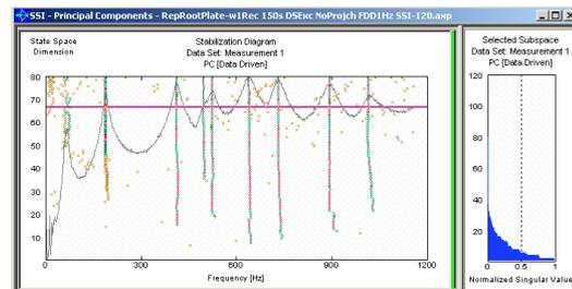
**Figs.10a** Stabilization diagram with two fixed broadbanded excitation sources
