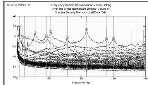
**Fig.3b** SVD plot from a test of the outer part of an airplane wing
