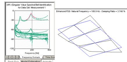
**Figs.5b** Torsion mode estimated from the FDD (SVD) shown in Fig 4b
