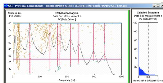
**Figs.10b** Stabilization diagram with two moving broadbanded excitation sources
