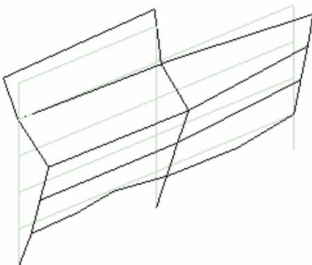
Figure 9: Mah Building Mode 1 – 2.334 Hz
