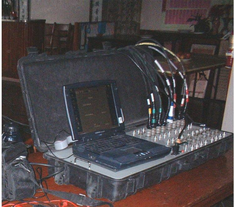
Figure 5: UBC EERF Data Acquisition System
