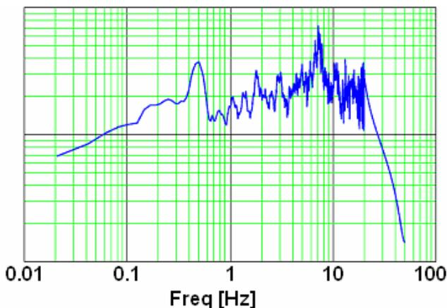
Figure 10: Normalized H/V Ratio, Test #1
