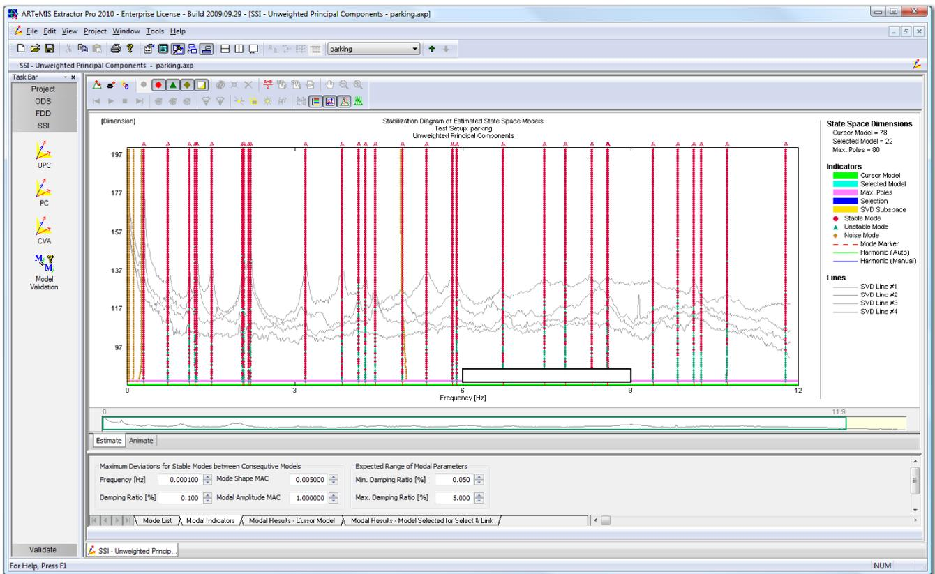
Figure 5: Stability diagram using Crystal Clear SSI<sup>®</sup> at the lower frequency range
