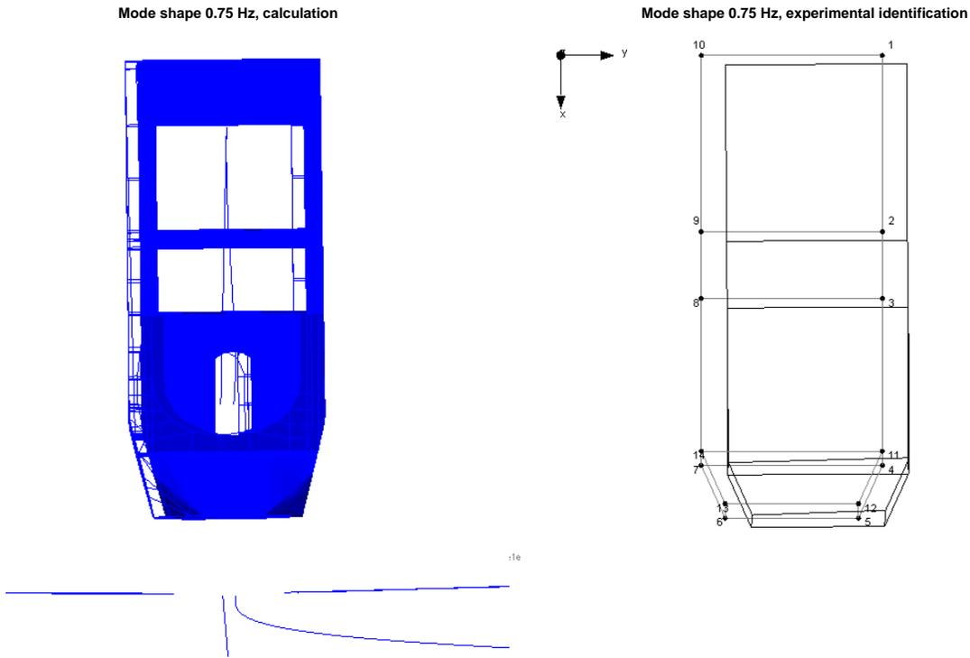
**Figure 10:** Mode shape identification using correlated modes: calculated flap wise (blades are pitched in feathered position) bending mode (left) and corresponding experimentally identified mode shape (right)
