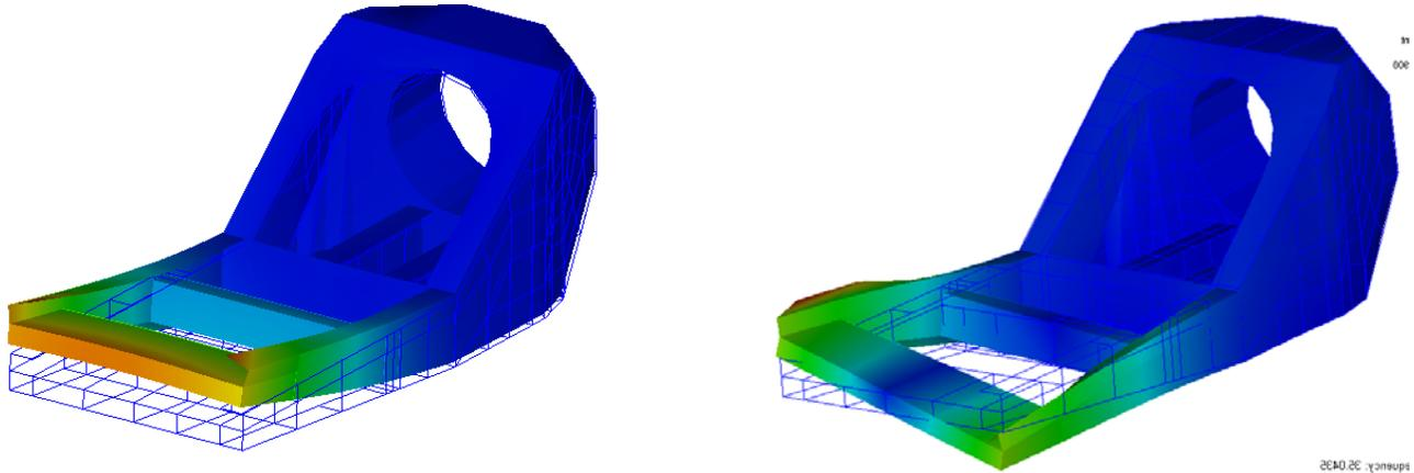
**Figure 12:** Calculated mode shapes based on the comprehensive wind turbine model
