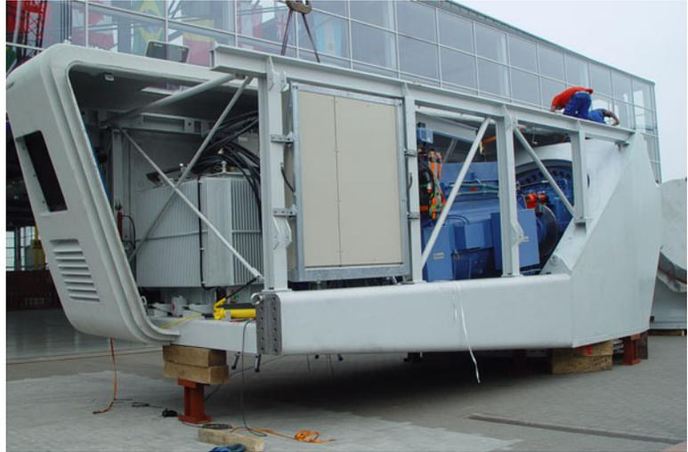
**Figure 2:** Nacelle construction with main frame
