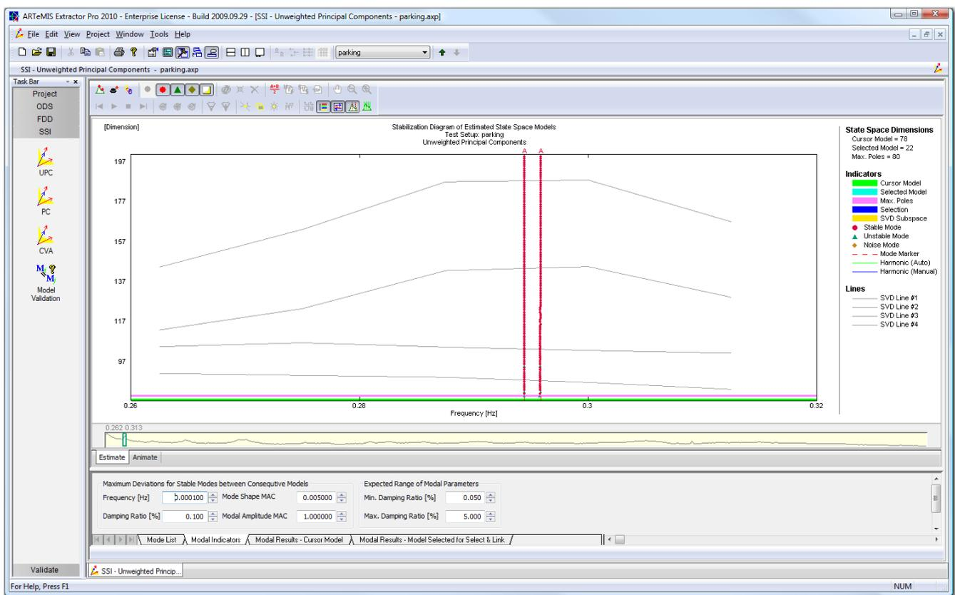
**Figure 7:** Separation and identification of repeated modes (first tower bending, perpendicular mode shapes)
