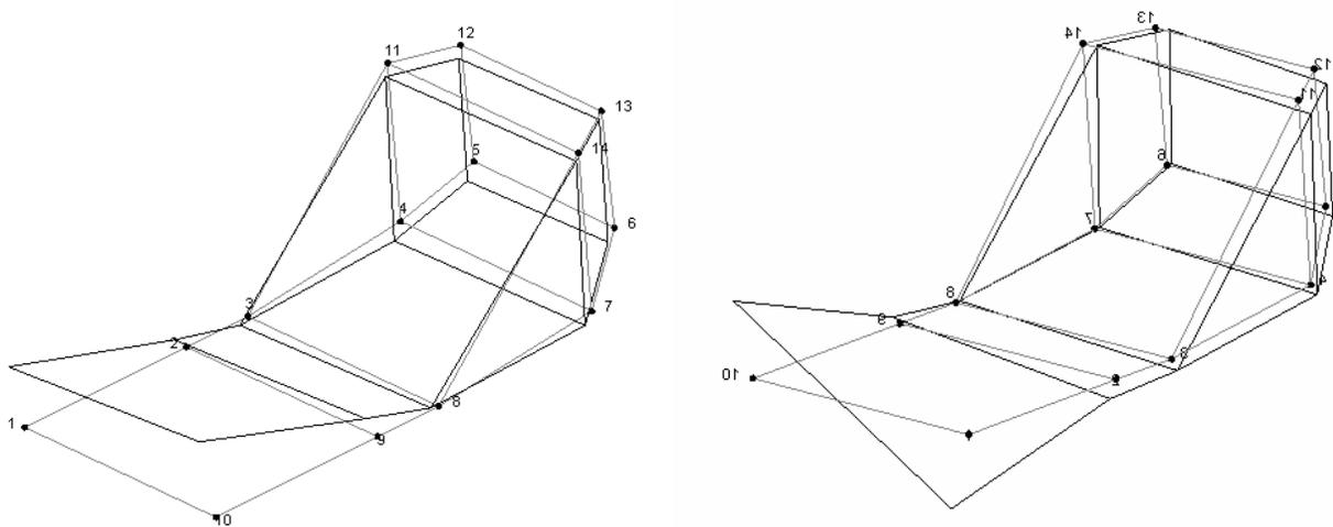
**Figure 11:** Experimentally identified mode shapes of the main frame, based on measurement data only
