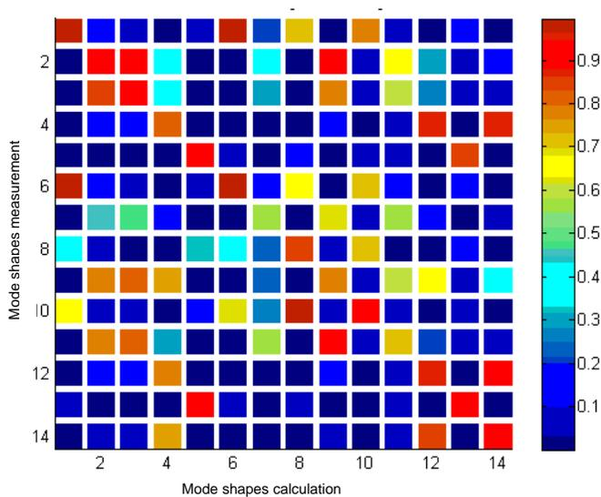
**Figure 9:** Application of Modal Assurance Criterion (MAC) to experimentally identified and calculated mode shapes
