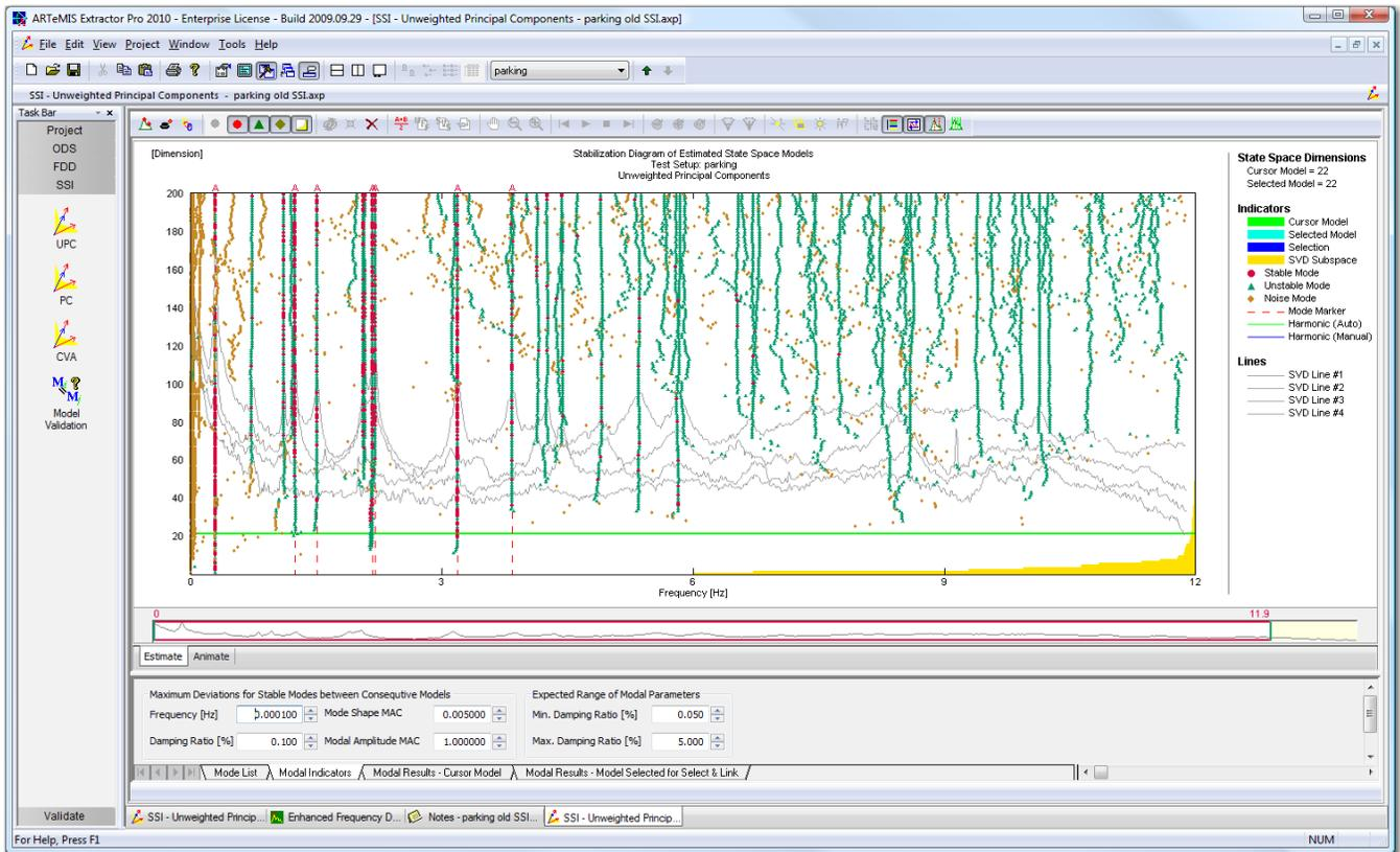
Figure 6: Stability diagram using standard SSI at the lower frequency range
