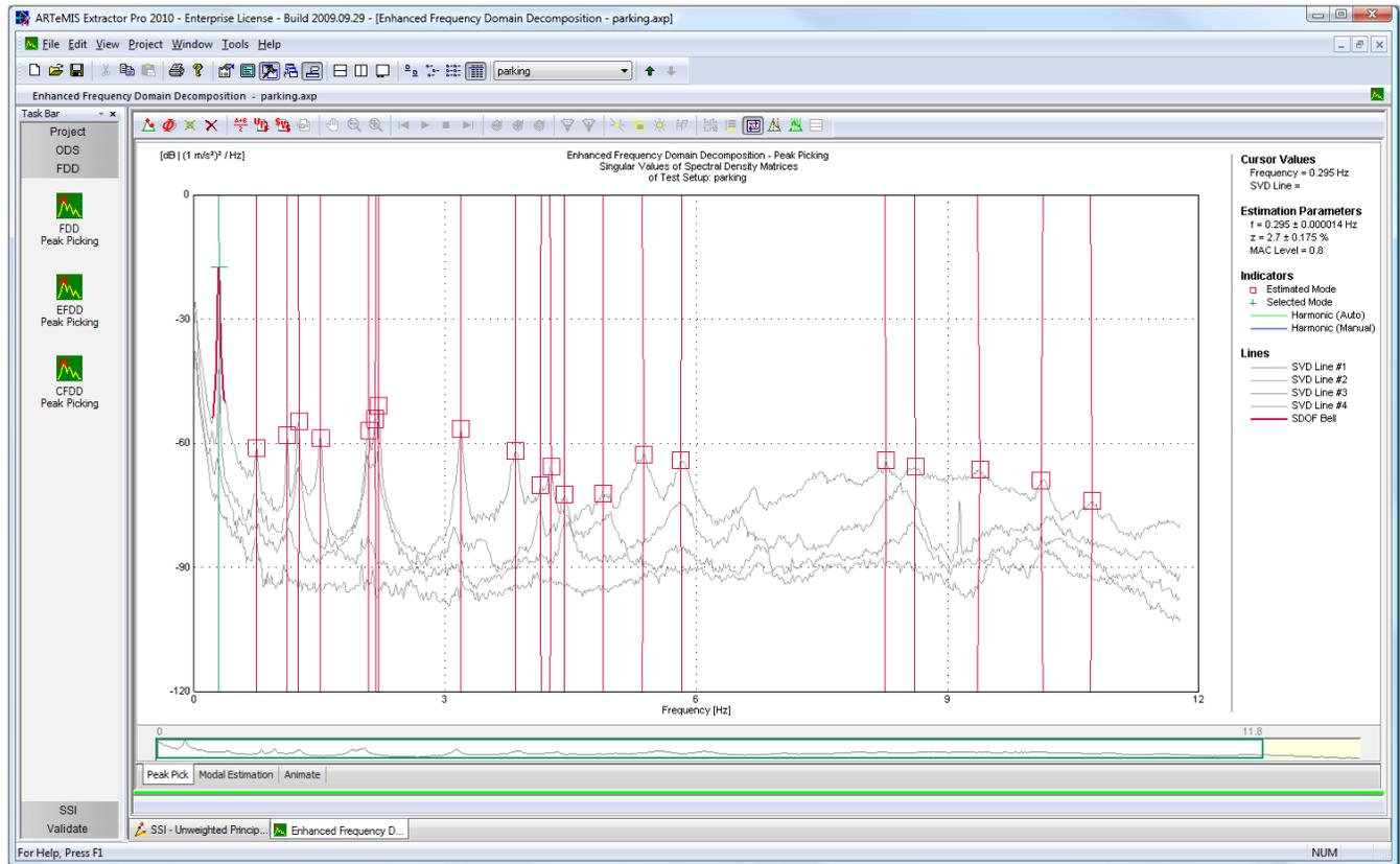
**Figure 4:** Singular values of spectral density matrices at the lower frequency range with selected spectral bell
