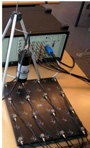
**Figure 2.** Test of a rectangular aluminum plate with 16 uni-axial accelerometers positioned in a 4 by 4 grid.
