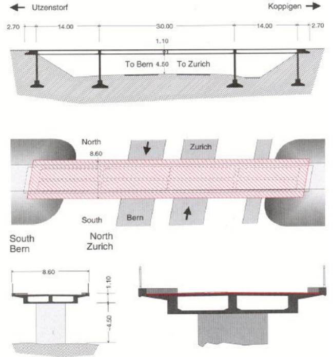
Figure 1: Schematic view of the Z24 Bridge.
