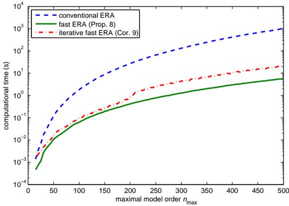
Figure 4: Computation times for multi-order ERA system identification of system matrices  $A_j$  and  $C_j$ ,  $n_j = j = 1, \dots, n_{\max}$  from  $O_{n_{\max}}$  at different maximal model orders  $n_{\max}$  with  $r = 251$ ,  $r_0 = 5$ ,  $c \approx 50$ .
