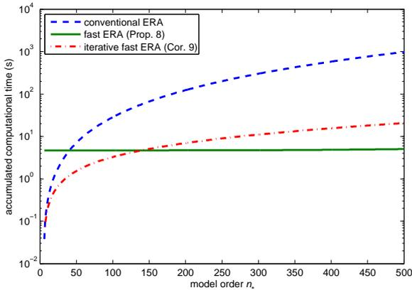
Figure 5: Accumulated computation times for multi-order ERA system identification up to different model orders  $n_*$  with maximal model order  $n_{\max} = 500$  and  $r = 251$ ,  $r_0 = 5$ ,  $c \approx 50$ .
