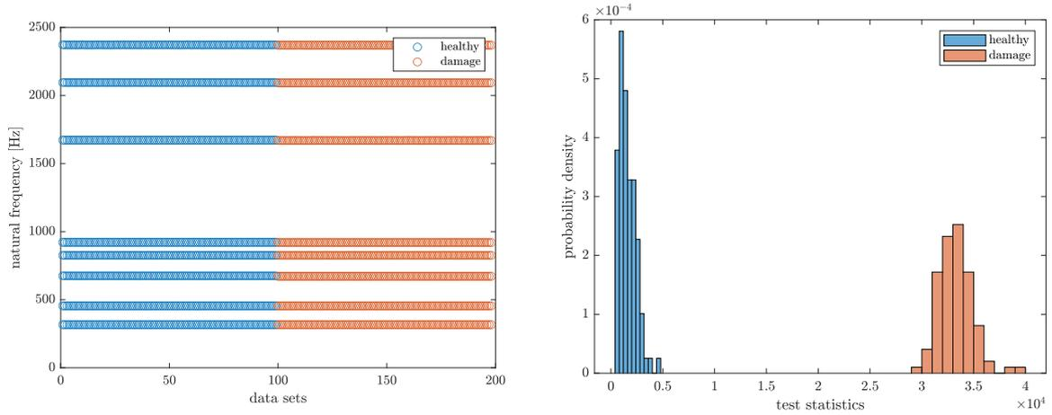
**Figure 3:** Natural frequency estimates obtained from both healthy and damage data (left). Histograms of damage detection test (right).
