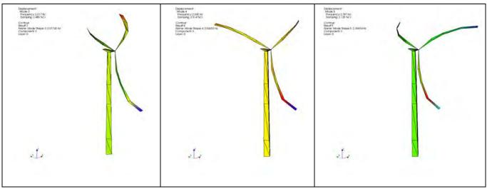
Figure 6. First three flapwise bending modes.
