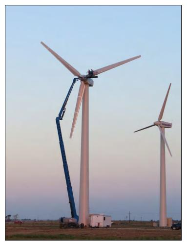
Figure 3. Impact modal testing performed on SNL1.
