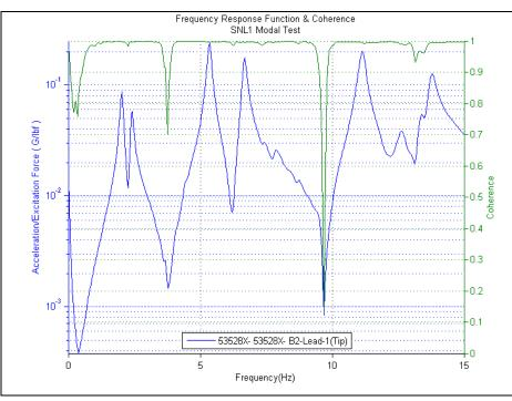
Figure 4. Drive point FRF and coherence from impact on SNL1 blade tip.
